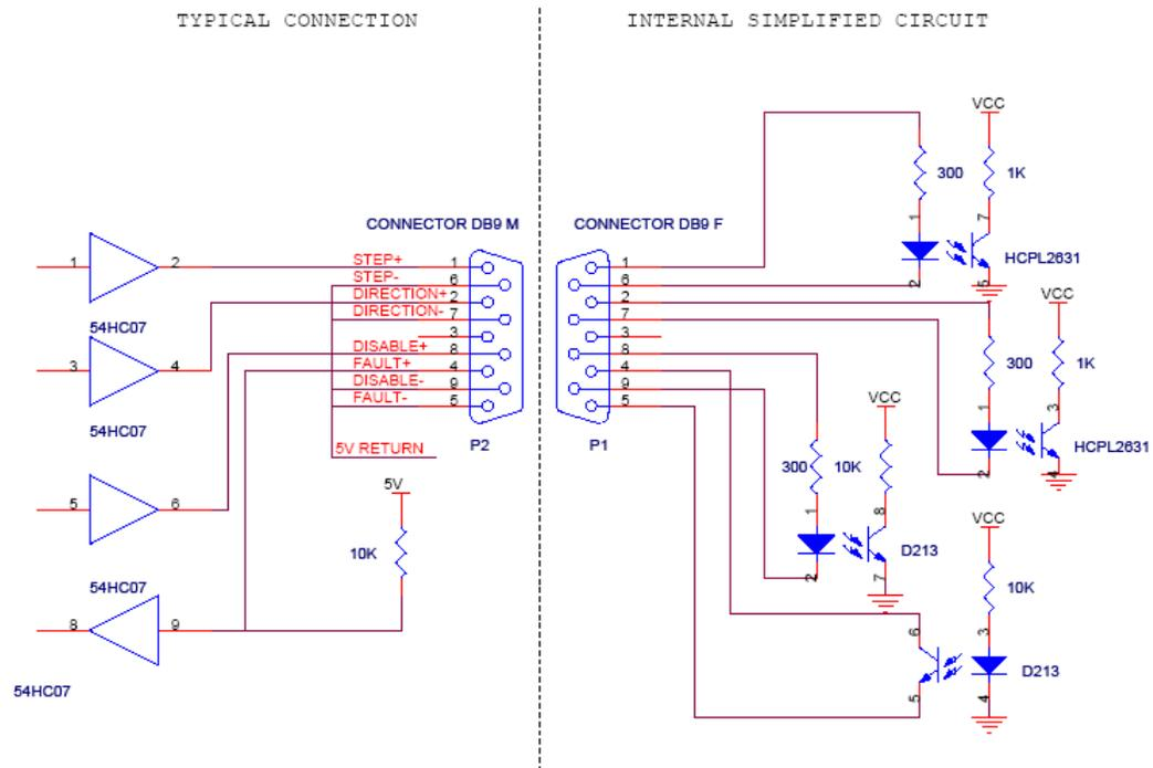
The STEP+, STEP-, DIRECTION+, and DIRECTION- signals are required for operation of the motor. These signals are photo-coupled to eliminate ground loops. The direction signal must not change 50 usec. prior to the step signal changing. A remote shutdown input is provided to remove power from the drive without removing DC power from the drive.
